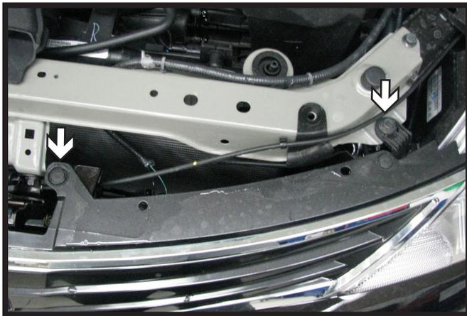
2. Remove the two (2) push pins from the top of the fascia. Do this on both sides of the vehicle.
